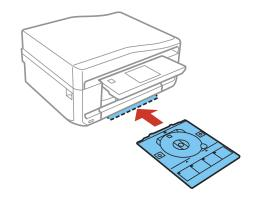
After printing, handle the CD or DVD carefully. You may need to wait up to 24 hours for the ink to dry fully before inserting it in a drive, depending on the type of disc you used. Keep printed discs away from moisture and direct sunlight.
